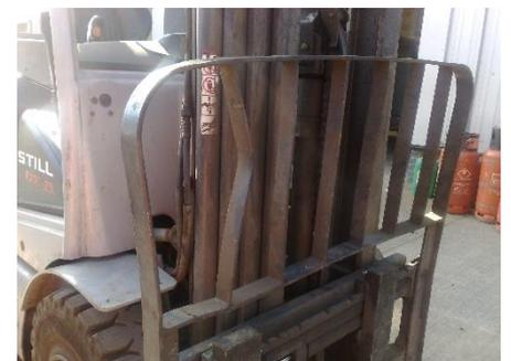
Lubrication — not usually required of a healthy forklift mast as it attracts detritus — could be a sign that the owner is compensating for a fault.
