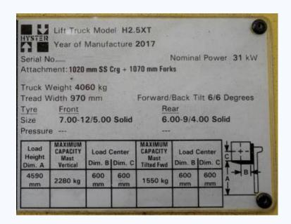
The above rating plate shows the load centres (Dim. B and C) and the load capacities of the fork lift truck with its mast in the vertical (2,280 kg) and tilted forward (1,550 kg) positions.
