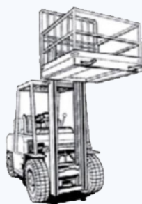
Figure 1 Counterbalance truck with non-integrated working platform
